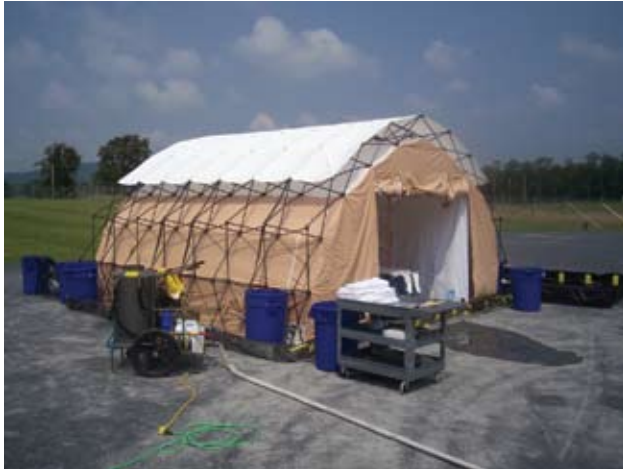
Fig. 16-5. TVI (TVI Corporation Inc, Glenn Dale, Md) decontamination pop-up shelter consisting of a light-weight scissor frame tent, integrated plumbing, heater, water bladder, and quickly expandable light-weight roller system with back-board. It can easily be erected within a few minutes by two individuals. Shown is a small size tent. Can be configured for both ambulatory and litter patients. Photograph: Courtesy TVI Corporation.
